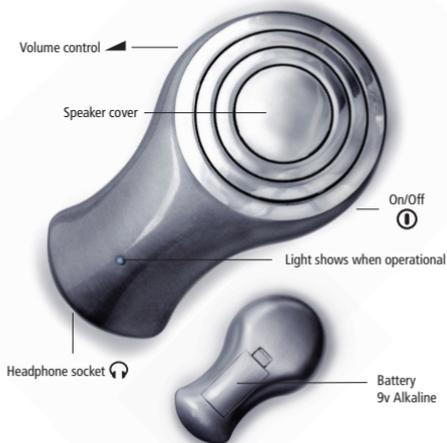
The Electrosmog Detector can identify the source, the source type and the intensity of your wireless microwave radiation.
